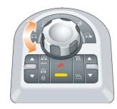
The Terrain Response system, if fitted, is always active and cannot be switched off. When the vehicle is started the system will normally start in its **General** program.
